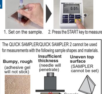
The QUICK SAMPLER/QUICK SAMPLER 2 cannot be used for measurements with the following sample shapes and materials.
