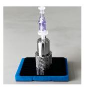
Set the Sampler on the enclosed sponge base when not conducting a measurement. Align the tip of the needle with the hole on the sponge base before setting the Sampler.
