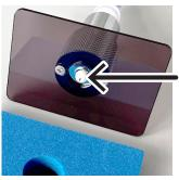
The tip of the needle protrudes slightly from the adhesive gel, so if the Sampler is set down without using the sponge base, the needle could bend and become unusable.
