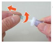
1. Remove the needle (NN-2116R) enclosed with the oxygen meter.
