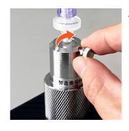
7. Turn the knurled screw clockwise to tighten it.
