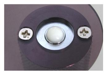
**3. Attach the new adhesive gel to the center section.** It takes about 30 minutes for the adhesive strength to appear after the gel is attached. When possible, wait at least 30 minutes before attaching the needle.
