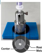
Set the Sampler on the enclosed sponge base when not conducting a measurement. Align the tip of the needle with the hole on the sponge base before setting the Sampler. (Note that the resin plate and metal section centers are deviated.)
