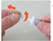
1. Remove the needle (NN-2116R) enclosed with the oxygen meter.
