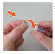
3. Attach the enclosed needle (NN-2138S) onto the fitting.
