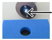
The tip of the needle protrudes slightly from the adhesive gel, so if the Sampler is set down without using the sponge base, the needle could bend and become unusable.
