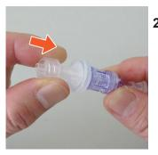
2. Attach the enclosed fitting onto the end of the membrane filter.
