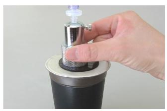
Set the resin plate section of the QUICK SAMPLER 2 onto the center of the sample. The adhesive gel will adhere under the weight of the Sampler , and the needle will pierce the packaging material. Follow the operation methods for the oxygen meter and conduct the measurement.
